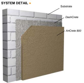
**SURFACE PREPARATION** • All bases should be sufficiently rigid, clean of any surface contamination that may prevent good suction. Dense, smooth surfaces, and those retaining excessive amount of form release agent can cause delamination of the plaster from the base. High gloss, or low absorption surfaces can be made more receptive by sandblasting.
