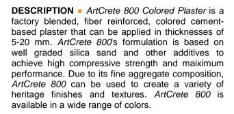
**USES** • ArtCrete 800 is an economical, yet higher performance alternative to a 3-coat dash coat - brown coat - paint system. ArtCrete 800 is typically applied on block work and concrete as the leveling and finish layer in a 2-coat system, replacing the need to install a gray plaster layer and a paint coating. ArtCrete 800 must be applied on a keying coat of DashCrete Splatter Dash Coat. ArtCrete 800 is suitable for interior and exterior applications and can be applied by hand or by machine.
